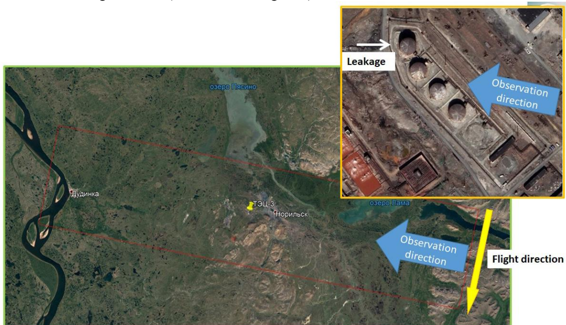
Figure 1. Image of TPP-3 area and geometry of Sentinel-1 SAR observation from descending orbit.
