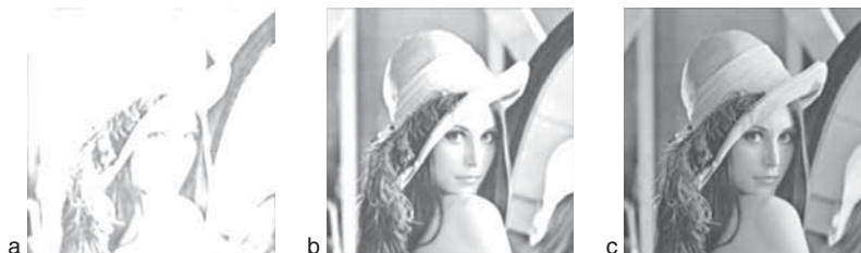
Figure 3. The simulation results of image «Lena» with using filter F_1 and different degrees n : a) n=4, PSNR=6,22 ; b) n=6, PSNR=12,09 ; c) n=8, PSNR=24,69
