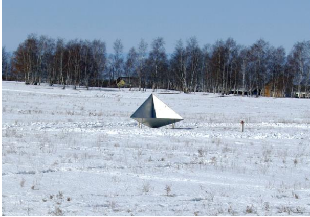
Fig. 3 Trihedral corner reflector on the test field.
