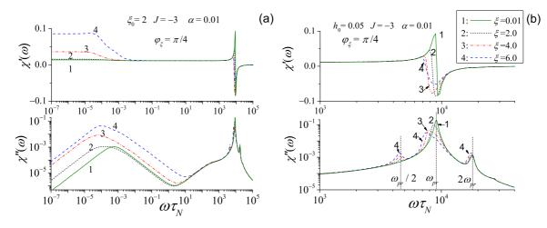
FIG. 4. (Color online) (a) Real and imaginary parts of the nonlinear susceptibility  $\text{Re}[\chi(\omega)]$  and  $-\text{Im}[\chi(\omega)]$  vs  $\omega\tau_N$  for various ac field amplitudes  $\xi$  and J = -3,  $\varphi_{\xi} = \pi/4$ ,  $\sigma = 20$ , and  $\xi_0 = 2$  using the matrix continued fraction solution. Solid lines: Linear response. Dashed lines: Nonlinear response. (b) The high-frequency parts of the spectra alone.
