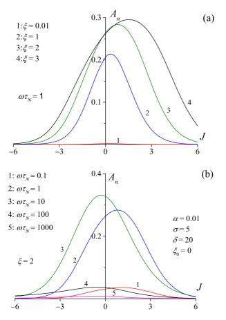
FIG. 10. (Color online) *Normalized* area of the DMH loop  $A_n$  [Eq. (12)] vs spin-polarized current parameter J (a) for various ac field amplitudes  $\xi$  and  $\omega \tau_N = 1$  and (b) for various frequencies  $\omega \tau_N$  and  $\xi = 2$  with  $\varphi_{\xi} = 0$ ,  $\alpha = 0.01$ ,  $\xi_0 = 0$ , and  $\sigma = 5$ .
