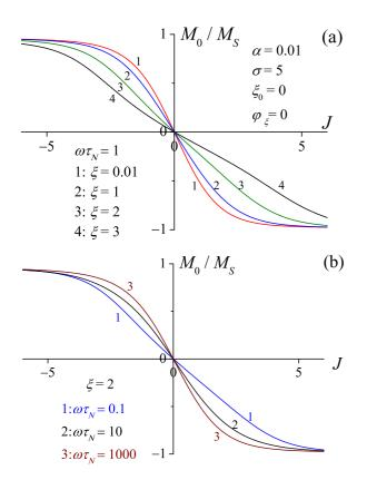
FIG. 3. (Color online) (a) Time-independent (dc) component of the magnetization  $M_0/M_S$  vs the spin-polarized current parameter J for (a) various ac field amplitudes  $\xi = 0.01, 1, 2$ , and 3 ( $\xi =$ 0.01 represents linear response) and  $\omega \tau_N = 1$  and for (b) various dimensionless frequencies  $\omega \tau_N = 10^{-1}$ , 10, and  $10^3$  at  $\xi = 2$  at  $\sigma = 5$ ,  $\varphi_{\xi} = 0$ , and  $\xi_0 = 0$ .
