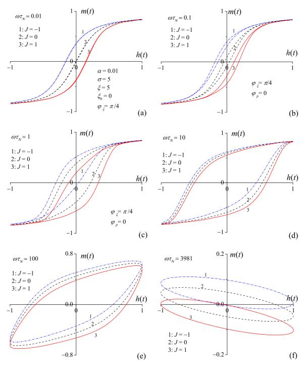
FIG. 9. (Color online) DMH loops for various spin-polarized current parameters J = -1, 0, 1 and frequencies  $\omega \tau_N = 10^{-2}$  (a),  $10^{-1}$  (b), 1 (c), 10 (d),  $10^2$  (e), and 3981 (f) with  $\varphi_{\xi} = \pi/4, \alpha = 0.01, \xi_0 = 0, \xi = 5$ , and  $\sigma = 5$ .
