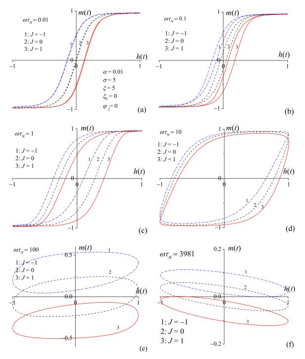
FIG. 8. (Color online) DMH loops for various spin-polarized current parameters J = -1, 0, 1 and frequencies  $\omega \tau_N = 10^{-2}$  (a),  $10^{-1}$  (b), 1 (c), 10 (d),  $10^2$  (e), and 3981 (f) with  $\varphi_{\xi} = 0, \alpha = 0.01, \xi_0 = 0, \xi = 5$ , and  $\sigma = 5$ .
