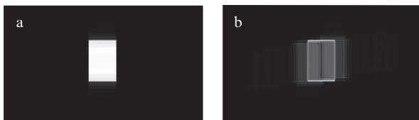
Figure 3. (a) Original image and (b) its appearance after FFT processing using the selected region in Fig. 2 as a spatial frequency filter.
