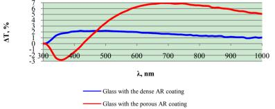
Figure 3. Change in optical transmittance of silica glass with the AR coatings in comparison with the uncoated glass.  $\Delta T = Tglass$  with the AR coating – Tglass without the AR coating.
