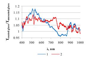
**Figure 6.** A ratio of the coated silica glasses (PMMA+Ag [3wt.%] thick films) transmission coefficient to uncoated silica glass transmission coefficient depending on  $\lambda$ . Film thickness: 1 - 35  $\mu$ m, 2 - 80  $\mu$ m.
