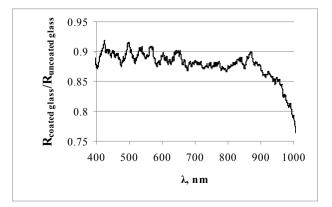
**Figure 5.** A ratio of the coated silica glass (PMMA+Ag [3 wt.%] thick film) reflection coefficient to uncoated substrate reflection coefficient depending on  $\lambda$ . Film thickness - 35  $\mu$ m.
