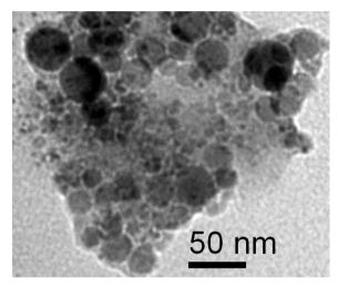
Figure 4. Scanning electron micrograph of silver NPs in PMMA.
