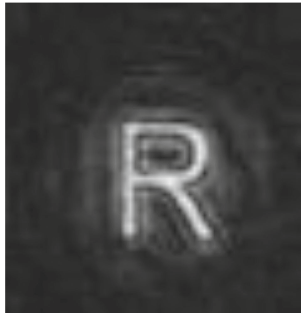
Fig. 6. Image of object “R” reconstructed by means of IF (5). The role of the IF is played by the hologram in Fig. 3, averaged over a ring.
