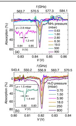
FIG. 3. Terahertz absorption signal vs voltage across the stack for different pressures of (a) ammonia vapor and (b) water vapor. The frequency displayed at the upper abscissa is calculated via the Josephson relation f = 2eV/hN, with N = 712. The inset in (a) shows the NH<sub>3</sub> absorption spectrum at p = 2.8 mbar, and the inset in (b) the H<sub>2</sub>O absorption spectrum at p = 1.5 mbar.
