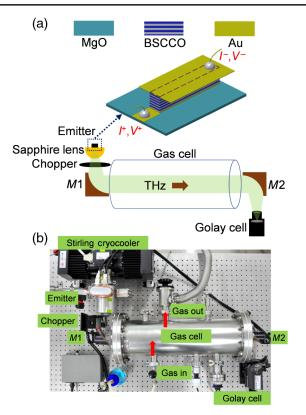
FIG. 1. (a) Sketch and (b) photograph of the terahertz gasdetection system with BSCCO intrinsic Josephson junctions as a tunable terahertz emitter. M1 and M2 denote parabolic mirrors. The IJJ stack forming a GBG structure is shown at the top of the sketch.
