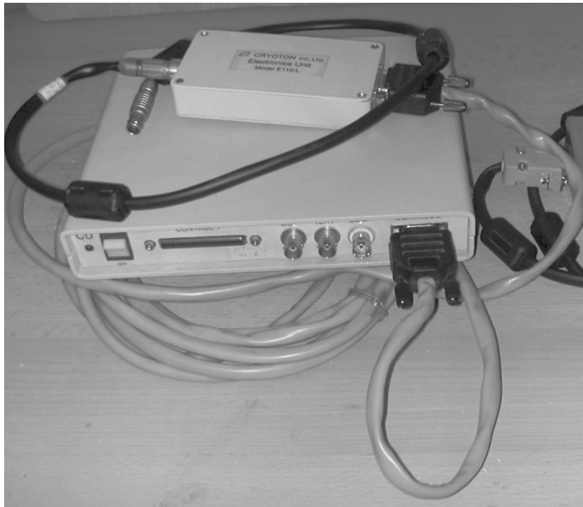
Fig. 4. Photograph of the SQUID electronics and control unit of the prototype of the single-channel SQUID gradiometer.
