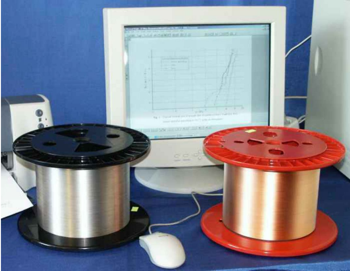
Figure 2. Metal coated optical fibers (aluminium and copper alloy).
