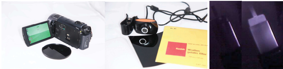
Fig. 3 Cameras and filters used in experiments (left) and the resulting image (for example the heated soldering hot air gun was used)(right).
