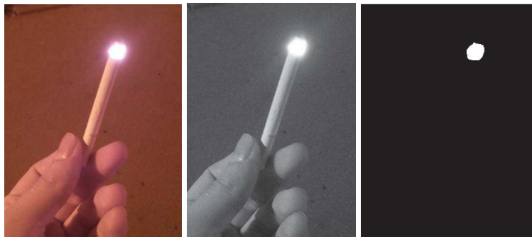
Fig. 6 An example of image processing with the webcam with a filter at the cigarette smoldering (the original image on the left preconditioning image in the center, highlighted contrasting object on the right).
