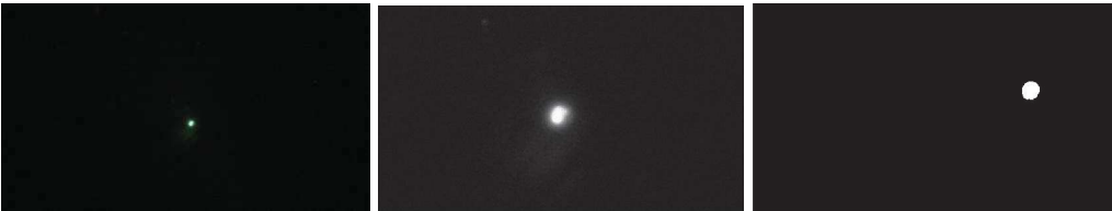
Fig. 5 An example of image processing with the Sony camera with a filter at the cigarette inhaling (the original image on the left preconditioning image in the center, highlighted contrasting object on the right).
