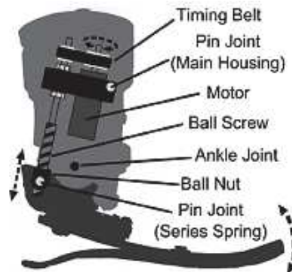
Fig. 1a prototype of Ankle–Foot Prosthesis with labeled components
