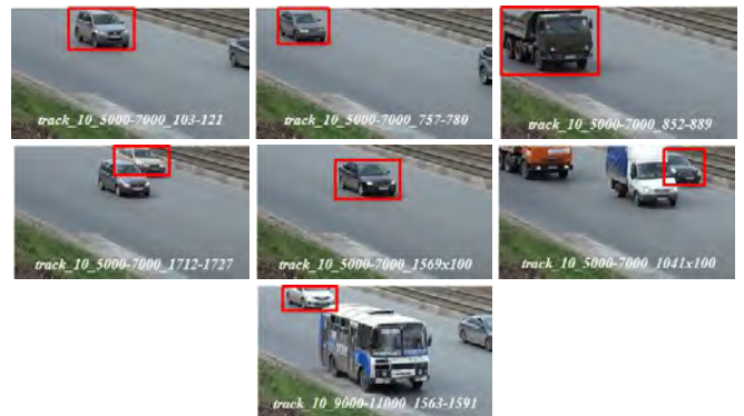
Fig. 5. The initial frames of test sequences for assessment of single vehicle tracking quality.
