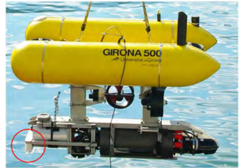
Fig. 6: The Girona500 AUV with the camera circled in red.
