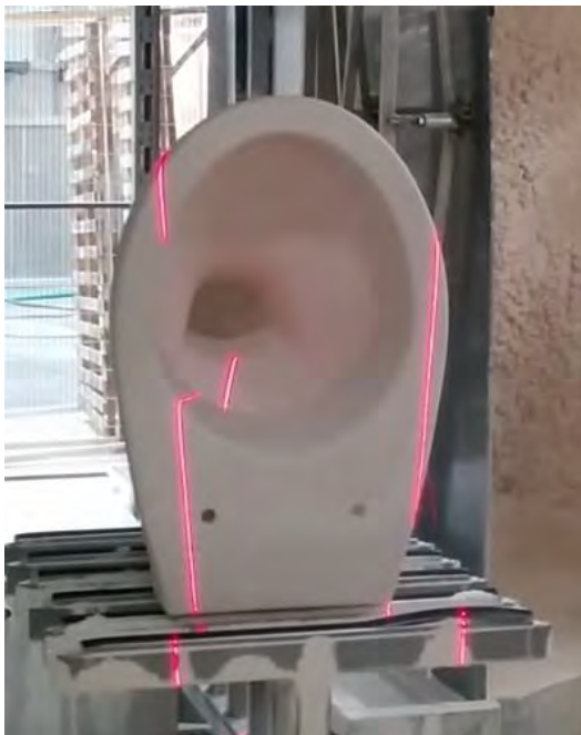
1 Figure 2: Workpiece with laser lines in the recognition stage
