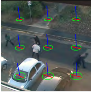
Fig. 4. An example of the computation of the characteristic distances in given positions of the ground plane. The green ellipse corresponds to the one meter diameter circle created around the position in the physical space. The red line corresponds to the characteristic distance, i.e., maximal diameter of the ellipse in the pixel space. The blue stick is an estimation of the vertical direction in the physical space.
