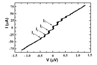
Fig. 1. *I-V* curve under external RF signal at frequency  $f_e$ =80 MHz Arrows point on positions of critical current  $I_c$  and Shapiro steps  $I_n$  for n= 1, 2, 3 at negative voltage biasing. Sample parameters:  $d_{SRO}$ =5.6 nm,  $d_{LSMO}$ =15 nm, L=50 µm,  $I_cR_n$ =0.22 µV.
