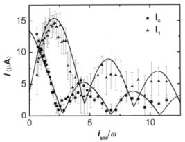
Fig.3. Amplitudes of critical current  $I_C$  and first Shapiro step  $I_I$  of the vs. normalized microwave current at  $f_e$ =3 GHz, T = 4.2 K and magnetic field H=133 Oe. Sample parameters:  $d_{SRO}$ =5.6 nm,  $d_{LSMO}$ =15 nm and L=50 µm,  $\lambda_r$ =220 µm. Solid lines show extended RSJ digital simulation for q=0.2.
