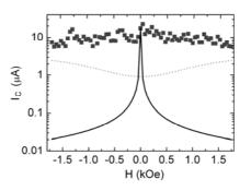
Fig. 4. Magnetic field dependence of critical current for a heterostructure with  $d_{SRO}$ = 8.5 nm,  $d_{LSMO}$ =3 nm, L=10 µm,  $\lambda_J$ =51 µm, measured in wide range of span. Dashed line shows noise floor. Solid line shows expected decay of maxima of  $I_C$  amplitudes oscillating by Fraunhofer dependence.
