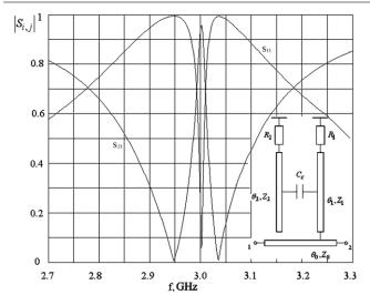
**Figure 1.** Frequency dependences of matrix parameters  $S_{11}$  and  $S_{21}$  calculated for a model of a meta-atom for the case  $C_c = 0.08 \text{ pF}$ ,  $Z_2 = 200 \Omega$ ,  $\theta_2 = 170^\circ$ ,  $\Delta \theta_2 = 10^\circ$ ,  $R_1 = R_2 = 5 \times 10^5 \Omega$  and  $f_2 = 2.84$  GHz. The circuit of the meta-atom is presented in the inset.
