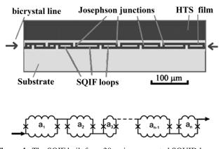
**Figure 4.** The SQIF built from 30 series-connected SQUID loops with areas in the range  $a_i = 50-400 \ \mu m^2$ . The width *w* of the Josephson junctions is 10  $\mu$ m. The top shows a zoom view of the bottom layer with a part of the SQIF. The equivalent circuit with the SQIF is shown at the bottom. Arrows indicate the bicrystal line.
