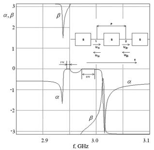
**Figure 6.** Frequency dependences of  $\beta$  and  $\alpha$  for the parameter  $\theta = \beta + i\alpha$ . The bandwidths of forward waves (FW) with positive  $\beta$  and backward waves (BW) with negative  $\beta$  are marked. Inset shows
