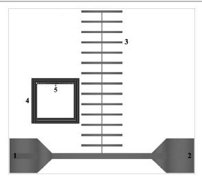
**Figure 3.** Thin film topology of the meta-atom on a NdGaO<sub>3</sub> substrate. 1 and 2 are the input/output ports of the microwave strip line, 3—radiating resonator ('electric dipole'), 4—spiral superconducting resonator with SQIF ('magnetic dipole'), 5—indicates the SQIF position.
