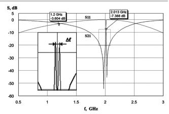
**Figure 5.** Simulated parameters  $S_{21}$  and  $S_{11}$  for the meta-atom, shown in figure 1. Inset shows two positions (a frequency shift) of the resonance peak of  $S_{21}$  marked by a rectangle. The  $\Delta f = 54$  MHz change in the resonance frequency corresponds to the case when the total inductance of the Josephson junctions in the SQIF has changed by 27 pH.
