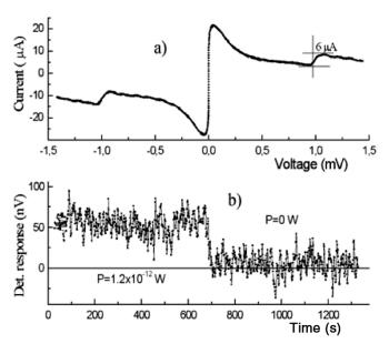
Fig. 6. Calibration of absorbed power and radiometric measurements at f = 500 GHz, T = 80 K a)—Josephson part of reduced *IV*-curve  $(I(V) - I \cdot (R_N)$  with Shapiro steps which allow us to estimate the power absorbed by the junction at high signal levels. b)—noise trace at low signal-to-noise ratio for known absorbed power. The NEP is estimated to  $6 \cdot 10^{-13} \text{ W/ Hz}^{1/2}$ .
