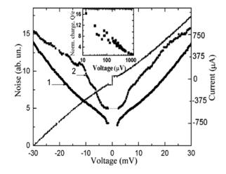
Fig. 5. The *I*-V curve and noise power  $P_N(V)$  in the 1–2 GHz frequency band (curve 1), and the 3–300 kHz band (curve 2) for a BJJ on sapphire substrate at T = 4.2 K. Inset: noise/current ratio in terms of effective transferred charge q(V) for bias voltages V < 1 mV.
