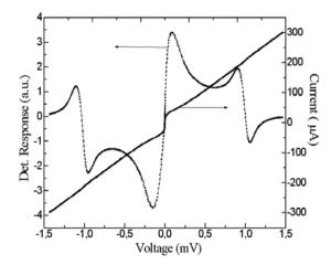
Fig. 2. Detector response of bicrystal Josephson junction on NdGaO<sub>3</sub> substrate for T = 80 K. An external 500 GHz radiation was applied. The response has two distinct features: first is the wideband response at low voltages and second is the frequency selective response at voltage  $V = h f_e/(2e)$ .
