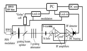
Fig. 1. Block diagram of set-up. The BWO is a submm wave source f = 220-550 GHz or 800–900 GHz. The PIN modulator is specially designed for the THz frequency range. The beam splitter is made from a metallic net. For simplicity the set of Teflon lenses is shown as one. The Golay cell is a submm wave detector. The Si hemispherical lens has diameter d = 12 mm and extension 3 mm. The JJ indicates the substrate with the BJJ and the integrated antenna.
