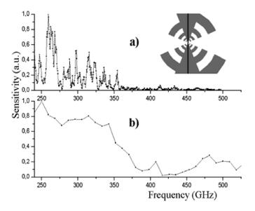
Fig. 3. Amplitude-frequency characteristics for a log-periodic antenna with a BJJ on sapphire at T = 20 K. (a) a metal (platinum) antenna was used, (b) all HTSC sample, evaluated by use of Fourier Transform Spectrometer.
