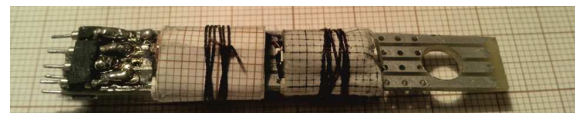
Fig.2. The appearance of the textolite framework with Gd samples for direct \Delta T and \Delta Q measurements in Bitter coil magnet.
