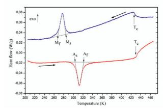
Figure 5. Differential scanning calorimetry scans. Ms, Mf and As, Af denote start and finish temperatures of the direct and reverse martensitic transformations, respectively.  $T_C$  – the Curie temperature of austenite.
