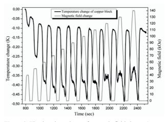
**Figure 8.** The time dependence of magnetic field change (gray curve) and a corresponding temperature change (black curve) of the copper block. The initial temperature is 273 K.
