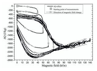
**Figure 9.** The dependence of  $\Delta Q$  on the magnetic field (black curve). The gray arrows show the direction of the magnetic field change. Gray square shows starting point of the measurements. The initial temperature is 273 K.
