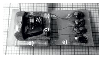
**Figure 7.** The appearance of the experimental setup for direct  $\Delta Q$ -measurements of MCE materials: a) the sample, b) the copper block, c) the diode for temperature measuring, d) the paper, e) the textolite framework.
