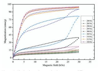
**Figure 2.** The isothermal magnetization curves at different temperatures, showing the magnetic-field-induced martensitic transformation.
