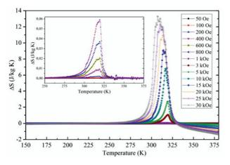
Figure 4. The calculated entropy change curves for the whole experimental magnetic field range of the ZFC protocol.
