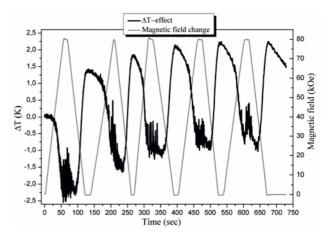
**Figure 6.** The time dependence of magnetic field change (gray curve) and the corresponding  $\Delta T$  (black curve) of the sample at adiabatic conditions. Initial temperature is 273 K.
