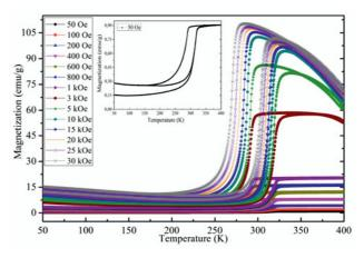
**Figure 3.** Thermo-magnetization curves at different fields, showing the shift of the martensitic transformation under applied magnetic field.
