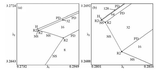
FIG. 5. Structure of bifurcation lines of Eq. (1) at b = 0.7. PD denotes period-doubling line, NS – line of Neimark-Sacker bifurcation, R2 – resonance 1:2 point, H – location of the critical point of H type. Numbers denote the period of the stable regime in the corresponding area.
