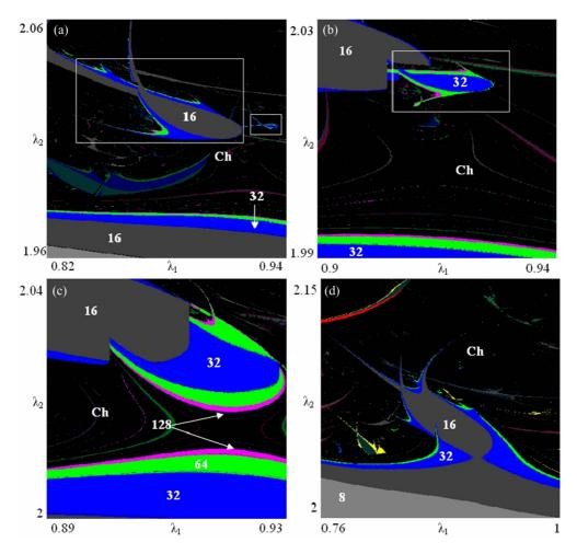
FIG. 6. (Color online) Fragments of the parameter plane illustrating the process of the formation of the Feigenbaum line rupture.  $\varepsilon = 0.4$ , *b* values: (a) 0.31, (b) 0.316, (c) 0.3215, and (d) 0.334. Color code as in Fig. 1. For better representation the period-32 window is shown fully, while from the period-16 window one part is cut out, since this part would overlay the period-32 window. Both attractors, period-16 and period-32, coexist and possess different basins of attraction.
