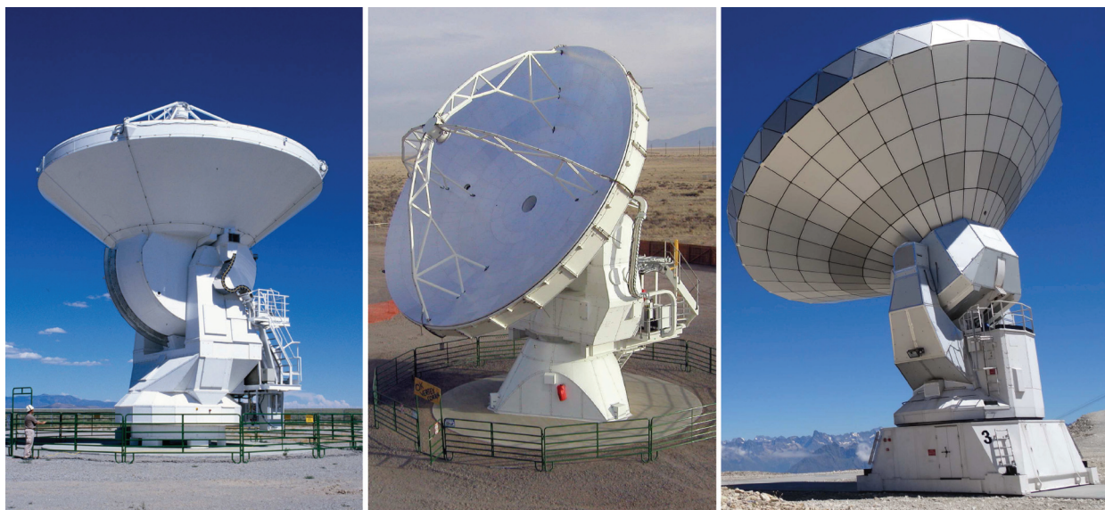
Fig. 4. Options of antennas for installation: (a) EIE antenna, credit: ALMA (ESO/NAOJ/NRAO); (b) Vertex antenna, credit: ALMA (ESO/NAOJ/NRAO); (c) NOEMA interferometer antenna, credit: NOEMA (IRAM).
