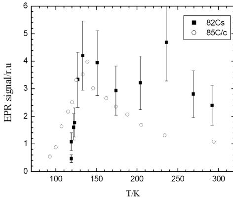
Fig.2. Temperature dependence EPR amplitude for two CSCO films with  $x=0.15$
