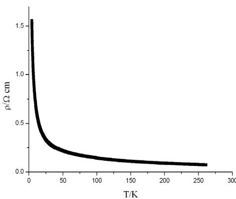
Fig.1. Temperature dependence of CSCO film resistance  $x=0.15$ .
