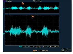
Fig. 6. Chaotic radio pulse sequence (upper plot) and its zoom fragment (lower plot).
