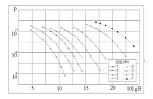
Fig. 3. Error probabilities *P* of noncoherent receiver as functions of processing gain at different SNR.
