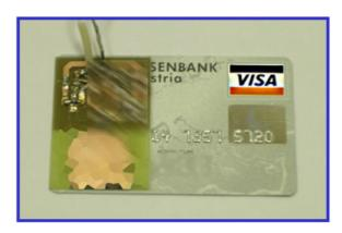
Fig. 4. Testbed of a small-size transmitter against a credit card
