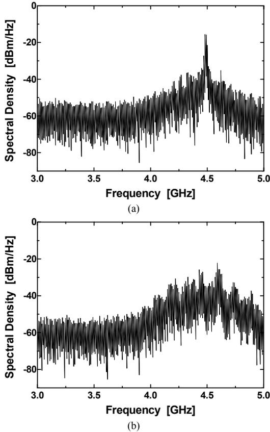
Fig. 8 Variable chaotic signal spectrums at  $f_c = 4.5$  GHz with (a) min. BW and (b) max. BW.
