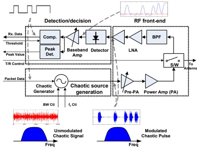
Fig. 1 System architecture and operation of the proposed flexible chaotic UWB communication.
