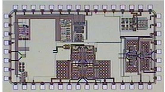
Fig. 12 Microphotograph of the CMOS RFIC for the flexible chaotic UWB system.
