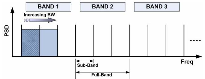
Fig. 2 Channel allocation in the flexible chaotic communication system with adjustable bandwidth.
