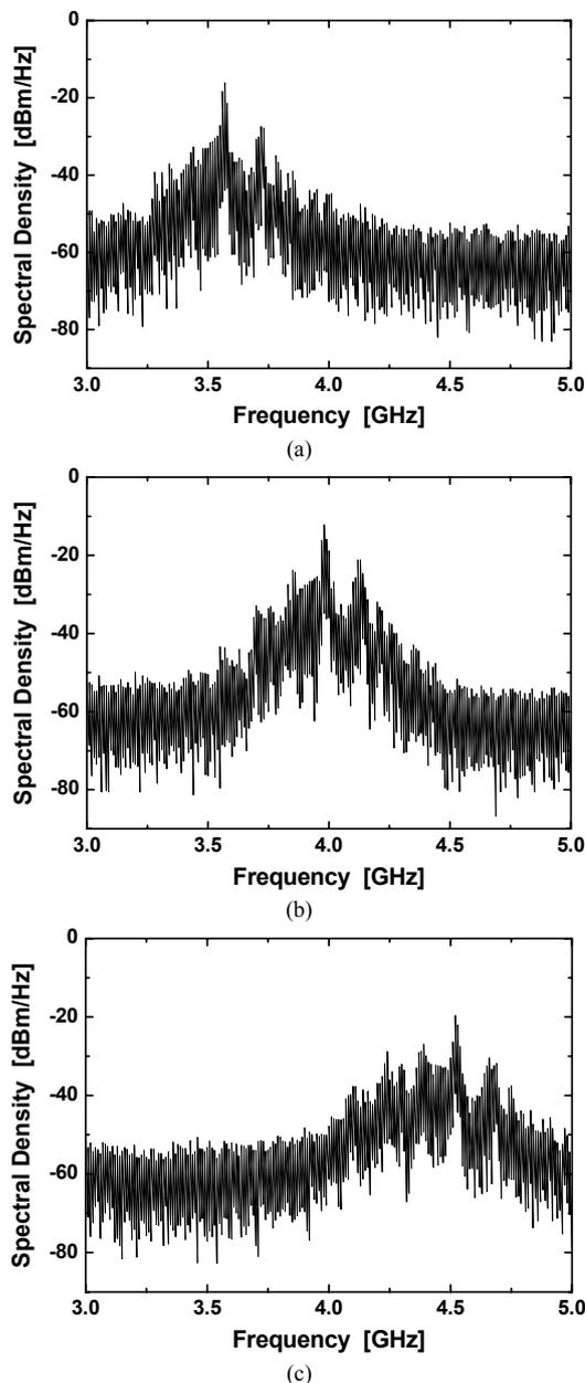
Fig. 7 Chaotic signal spectra for RF channels. (a) Channel 1 ( $f_c = 3.5$  GHz). (b) Channel 2 ( $f_c = 4.0$  GHz). (c) Channel 3 ( $f_c = 4.5$  GHz).
