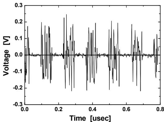
Fig. 9 Pulse-modulated chaotic signal waveform at the chaotic UWB transmitter output ( $R_s = 15$  Mbps,  $f_c = 4$  GHz, carrier BW = 500 MHz).
