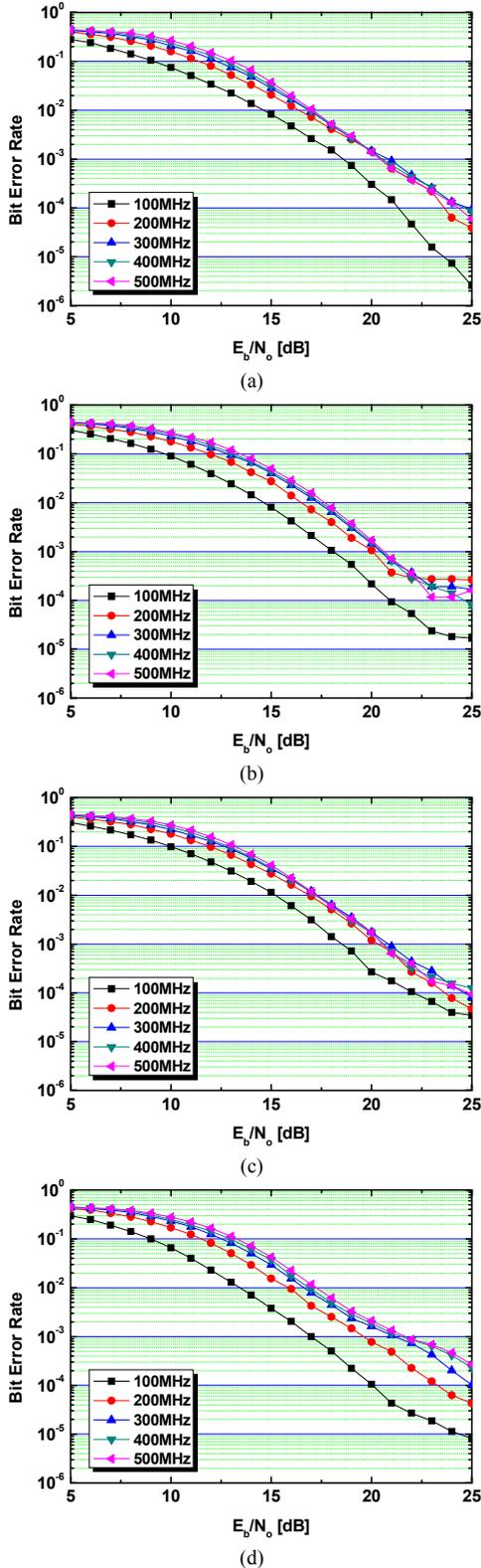
Fig. 3 System performance with various channel BWs for the following environments: (a) indoor residential LOS, (b) outdoor LOS, (c) industrial NLOS, and (d) agricultural area.
