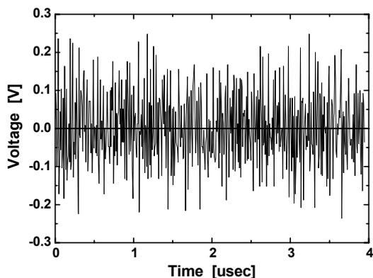
Fig. 6 Measured results of the chaotic signal waveform at  $f_c = 4$  GHz and BW = 500 MHz.
