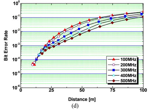
Fig. 4 Communication distance evaluation with various channel BWs for the following environments: (a) indoor residential LOS, (b) outdoor LOS, (c) industrial NLOS, and (d) agricultural area.
