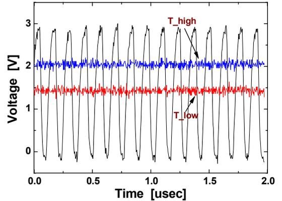
Fig. 10 Detected signal waveform at detector output of the chaotic UWB RFIC.
