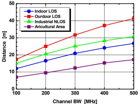
Fig. 11 Experimental results for communication distances corresponding to variable channel BWs.
