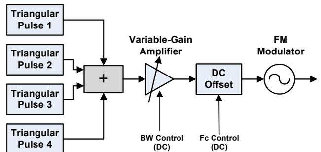
Fig. 5 Configuration of the flexible chaotic generator with variable center frequency and bandwidth.
