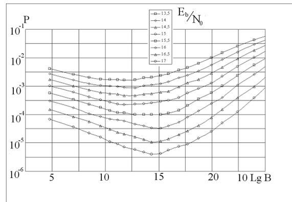
Fig. 2. Error probability  $P$  of noncoherent receiver as a function of processing gain  $B$  for different ratios  $E_b/N_0$ .
