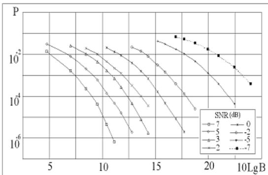
Fig. 3. Error probabilities  $P$  of noncoherent receiver as functions of processing gain at different SNR.
