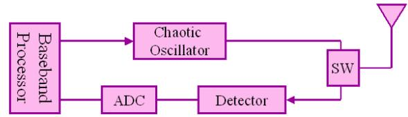
Fig. 1. The structure of WB and UWB Direct Chaotic Communications for low bit rate.
