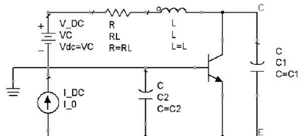
Fig. 2. Three-point scheme of generator. Representation in ADS.
