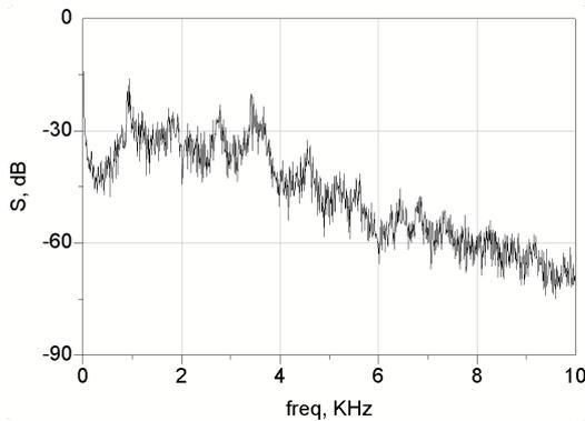
Fig. 7 (a). Power spectrum in three-point circuit with Gummel-Poon model of BFP620 transistor. Frequency range – kilohertz.  $\gamma = 2$ .
