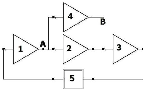
Fig. 4a. Block scheme of CMOS oscillator. 1, 2, 3 – amplifiers; 4 – output buffer amplifier; 5 – frequency selective circuit; A –point of signal taken from a feedback ring; B – out.
