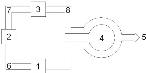
Fig. 2a. Block scheme of microstrip version of UWB microwave chaotic oscillator with distributed topology.
