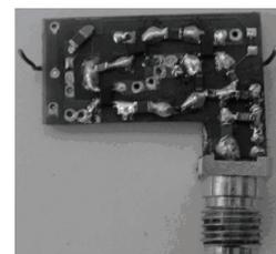
Fig. 3b. Experimental testbed of the UWB microwave chaotic oscillator with lumped elements.
