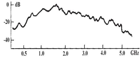
Fig. 2c. Typical chaotic oscillations power spectral density for oscillator with distributed topology (experiment).
