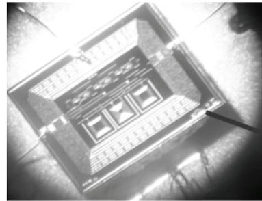
Fig. 4b. Experimental chaotic oscillator implementation as IC on the CMOS technology 180 nm.
