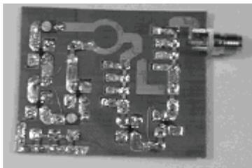
Fig. 2b. Experimental testbed of the microstrip version of UWB microwave chaotic oscillator with distributed topology.
