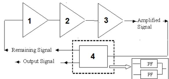
Fig. 3a. Block scheme of the UWB microwave chaotic oscillator with lumped FSC (PF –low or high pass filter).
