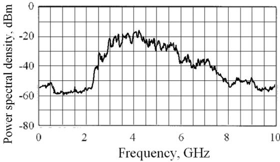
Fig. 3c. Typical chaotic oscillations power spectral density for oscillator with lumped elements (experiment).
