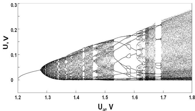
Fig.5. Single-parameter bifurcation diagram of oscillations modes.  $U_a$  – supply voltage,  $U$  – oscillations amplitude.
