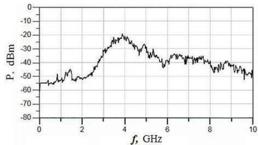
Fig. 4c. Typical chaotic oscillations power spectral density for 180nm CMOS oscillator with high frequencies FSC sections (modeling).
