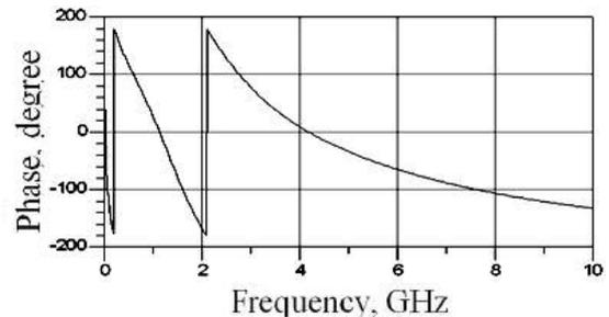
Fig.6. Phase frequency response of the oscillator feedback loop
