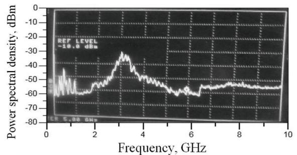
Fig. 4d. Typical chaotic oscillations power spectral density for 180nm CMOS oscillator with high frequencies FSC sections (experiment).
