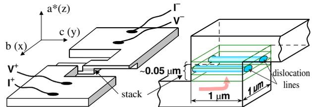
FIG. 1 (color online). Scheme of the tunneling device of type A. Crystallographic axes of NbSe<sub>3</sub>  $a^*$ ,  $b$ ,  $c$  ( $b$  is the chain direction) correspond to coordinates  $z$ ,  $x$ ,  $y$ . Elliptic cylinders show the cores of dislocation lines; the curved arrow shows the current path.
