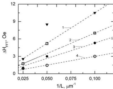
Fig. 5. Periods  $\Delta H_{FFT}$  of the Fourier components of  $I_C(H)$  dependences vs. parameter  $1/L$  for 3 heterostructures on a chip ( $d_{SRO}=8.5$  nm,  $d_{LSMO}=6$  nm) with widths  $L = 10$   $\mu\text{m}$ ,  $20$   $\mu\text{m}$ ,  $40$   $\mu\text{m}$ , having  $\lambda_J=120$   $\mu\text{m}$ ,  $110$   $\mu\text{m}$ , and  $190$   $\mu\text{m}$ , correspondingly. Harmonic numbers point on linear  $\Delta H_{FFT}(1/L)$  functions.
