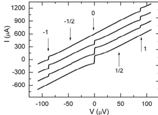
Fig. 2.  $I$ - $V$  characteristics under external microwave signal at  $f_e=40$  GHz, increasing microwave powers upwards. Arrows point on positions of critical current  $I_C$  ( $n=0$ ) and Shapiro steps  $I_n$  with integer  $n=\pm 1$ , and half-integer  $n=\pm 1/2$ .  $T=4.2$  K,  $H=0$ .
