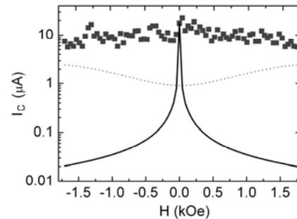
Fig. 4. Magnetic field dependence of critical current for a heterostructure with  $d_{SRO}=8.5$  nm,  $d_{LSMO}=3$  nm,  $L=10$   $\mu$ m,  $\lambda_J=51$   $\mu$ m, measured in wide range of span. Dashed line shows noise floor. Solid line shows expected decay of maxima of  $I_c$  amplitudes oscillating by Fraunhofer dependence.
