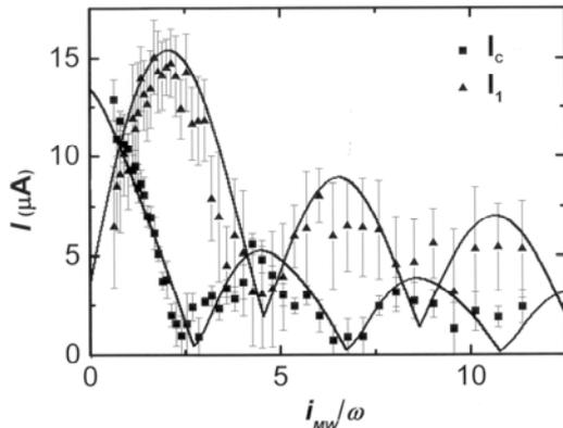
Fig. 3. Amplitudes of critical current  $I_c$  and first Shapiro step  $I_1$  of the vs. normalized microwave current at  $f_e=3$  GHz,  $T=4.2$  K and magnetic field  $H=133$  Oe. Sample parameters:  $d_{SRO}=5.6$  nm,  $d_{LSMO}=15$  nm and  $L=50$   $\mu$ m,  $\lambda_J=220$   $\mu$ m. Solid lines show extended RSJ digital simulation for  $q=0.2$ .
