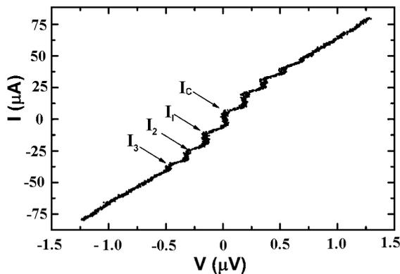
Fig. 1.  $I$ - $V$  curve under external RF signal at frequency  $f_e=80$  MHz. Arrows point on positions of critical current  $I_C$  and Shapiro steps  $I_n$  for  $n=1, 2, 3$  at negative voltage biasing. Sample parameters:  $d_{SRO}=5.6$  nm,  $d_{LSMO}=15$  nm,  $L=50$   $\mu$ m,  $I_C R_N=0.22$   $\mu$ V.
