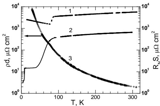
Figure 1. Temperature dependences of junction resistance: (1)  $d=20$  nm,  $S=10 \times 10 \mu\text{m}^2$ , (2)  $d=40$  nm,  $S=50 \times 50 \mu\text{m}^2$  and (3) resistance  $\rho d/S$  of a bare CSCO film with  $x=0.5$ ,  $d=40$  nm,  $S=50 \times 50 \mu\text{m}^2$  deposited on NGO substrate.
