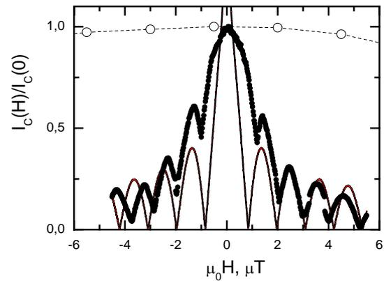
Figure 4. Magnetic-field dependence  $I_C(H)$  for structures with  $L = 50 \mu\text{m}$ . With AF interlayer - black points, and thin line is calculated curve by theory [4]. A central part for a structure without AF layer - open circles.
