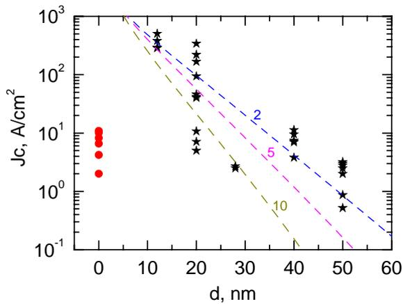
Figure 3. Thickness dependencies of critical current density for junctions with (and without at  $d=0$ ) AF interlayer. Dashes are theoretical dependences for S-AF-S junctions with different intensity of exchange field  $h$  (numbers) of F layers in AF.
