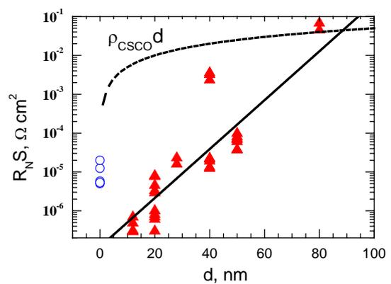
Figure 2. Thickness dependencies of specific resistance  $R_N S$  for CSCO with  $x=0.5$ . Bold line corresponds to  $\xi_{AF}=7 \pm 1$  nm. Open circles are data for junctions without AF interlayer. Dash line is calculated resistance for bare AF layer.
