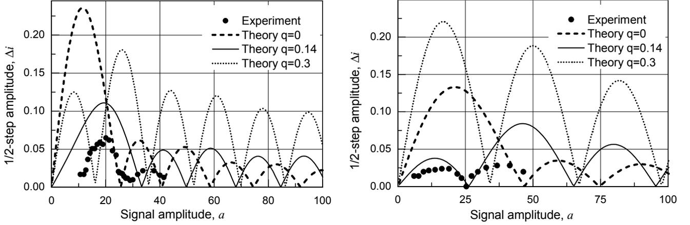
Fig. 2. Dependence of the 1/2-step amplitude  $\Delta i$  on the applied signal amplitude  $a$  at  $\beta = 4$  for frequencies  $\omega = 1.62$  (left side) and  $\omega = 2.2$  (right side). Dashed, solid and dotted lines correspond to the step behaviour given by formula (13) accordingly at  $q = 0$ ,  $q = 0.14$  and  $q = 0.3$ . The filled dots are experimental data for the  $c$ -tilted Nb/Au/YBCO junction.
