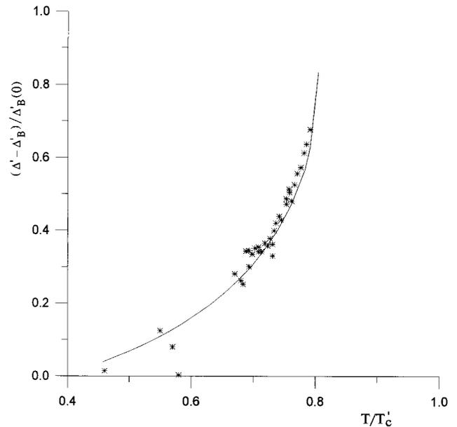
FIG. 3. The experimental temperature dependence of the deviation of the superconducting gap in the interlayer  $(\Delta')$  from the BCS theory one  $(\Delta' - \Delta_B)(T)$  for the SDBS J6N5 at  $V = V_+ = (\Delta + \Delta')/e$ . The solid line presents the calculated results for  $V = V_+$  at  $\tau_{in}(E) \approx \tau_{in0} \{ 1 + [\Delta' / (|E| - \Delta')]^{3.5} \}$ ,  $\Gamma \tau_{in} \approx 10^{-2}$ .
