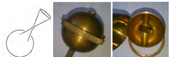
Fig. 4. Schematic view of back-to-back horn (a) and example of integrating cavity.
