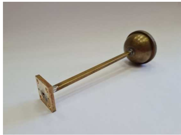
Fig. 4. Photo of the integrating cavity.
