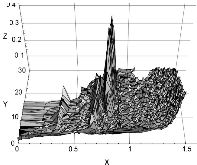
Fig. 6. Set of CRFFO I-V characteristics with detector 2 output signal shown in Z coordinate. Flux-flow is directed from detector 2. X coordinate is CRFFO bias voltage in mV. Y-coordinate is CRFFO bias current in mA. Z-coordinate is detector power a.u.
