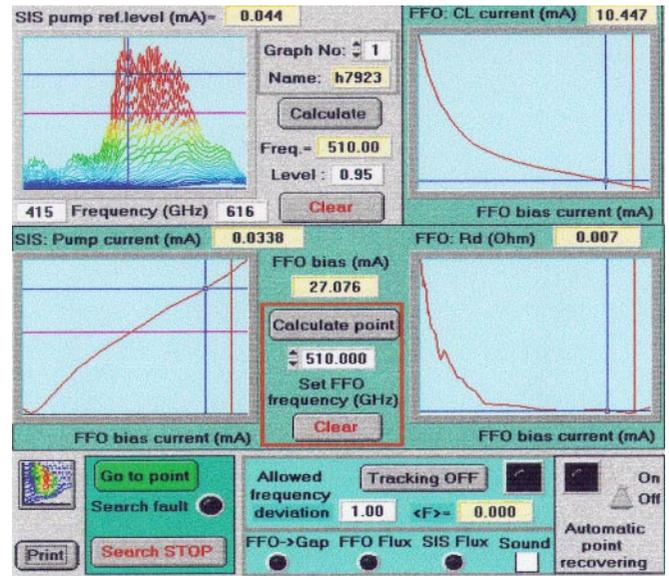
Fig.6. Panel of IRTECON showing data on pump efficiency of SIS mixer.
