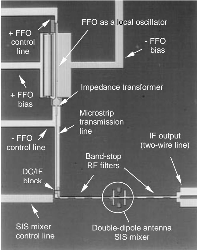
Fig. 1. Photograph of the chip receiver. The field of view is 1 mm x 1.5 mm.
