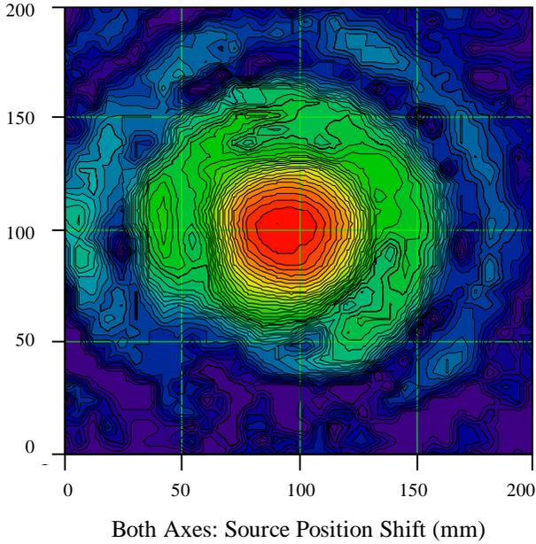
Fig. 2. Antenna beam pattern of reference SIS mixer; contour step is 1 dB.
