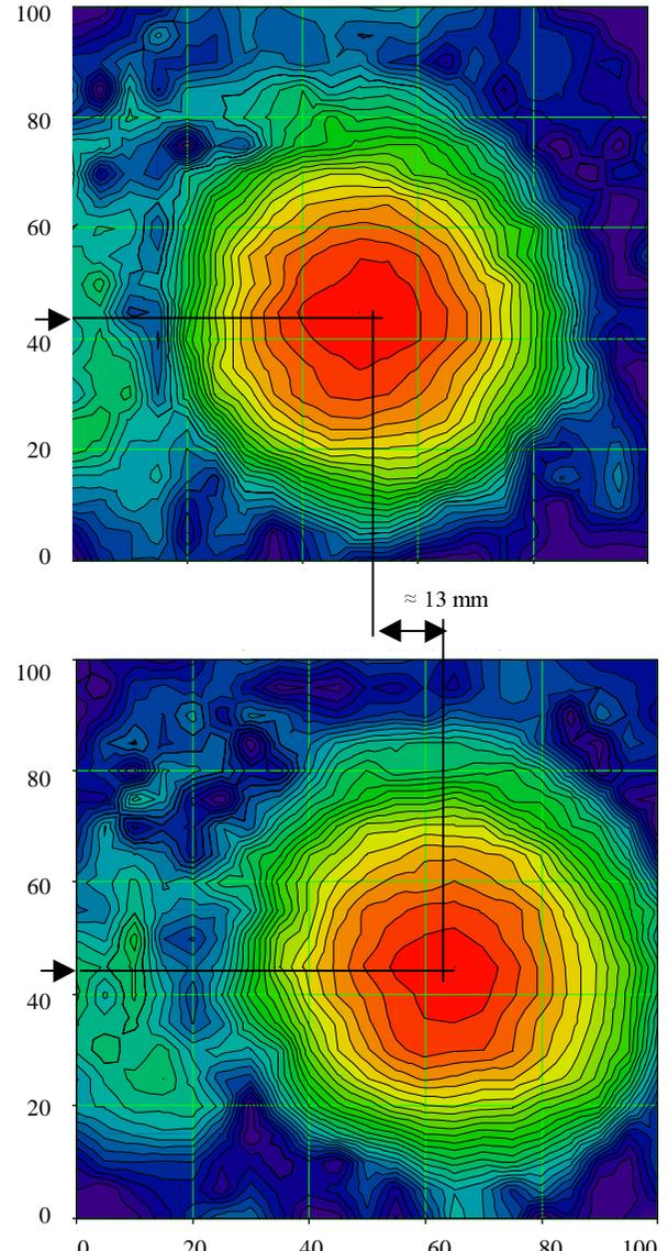
Fig. 3. Antenna beam patterns for two adjacent pixels; contour step is 1 dB. Both axes: source position shift (mm).
