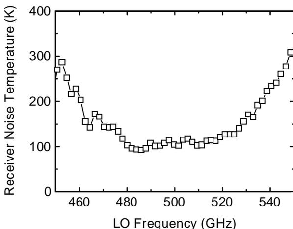
Fig. 5. Data on a pixel with balanced SIS mixer pumped by FFO in test cryostat.
