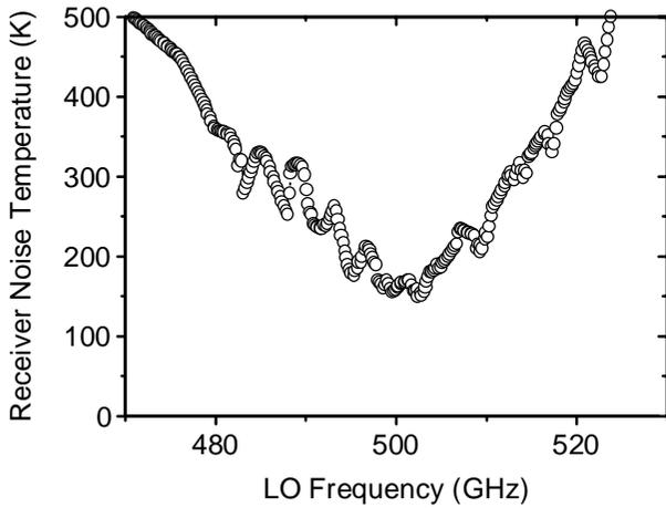
Fig. 4. Experimental data on a pixel with single-junction SIS mixer in the array dewar (pumped by internal FFO).
