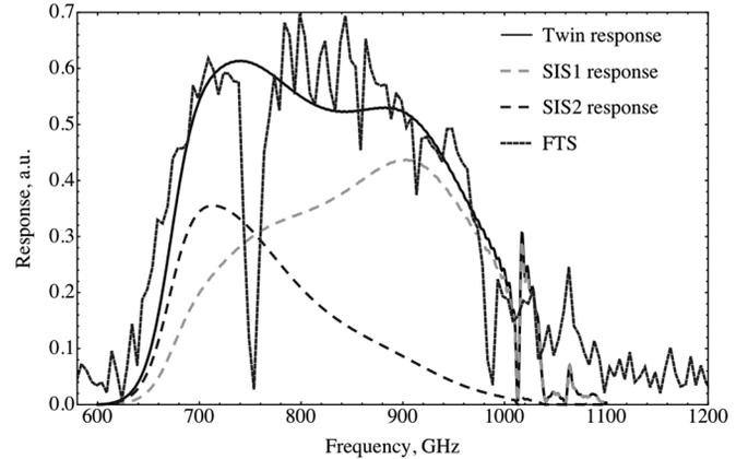
Fig. 2. Measured FTS response of the twin mixer—dotted line; simulations of the response—solid line; simulated response of each individual SIS mixer of the twin—dashed lines. Water vapour absorption lines are visible at 750 GHz and around 1 THz.
