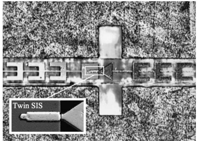
Fig. 1. Photograph of the SIS mixer (including the waveguide probe and filter structure) installed in a waveguide. The central part with SIS twin junction is magnified.
