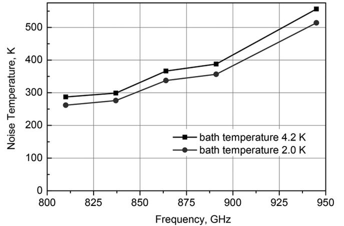
Fig. 5. DSB noise temperature, corrected for the beam splitter loss, measured at a bath temperature of 4.2 K (squares) and 2 K (circles).
