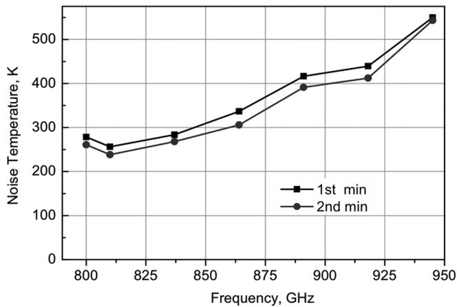
Fig. 3. DSB noise temperature, corrected for the loss in the LO insertion beam splitter, measured for the first (squares) and second (circles) minima of critical current suppression.
