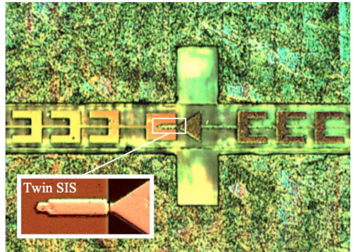
Fig. 1 Photo of the SIS mixer (including the antenna and the filter structure) installed in a waveguide. The central part with SIS twin junction is magnified.
