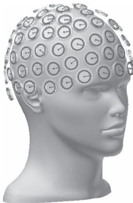
Fig. 7. Example of positioning more than 100 encapsulated HTM-D20 magnetometers around a 3D model of the head of an adult human.
