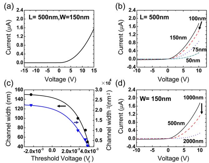
FIG. 2. (Color online) Pentacene in-plane diode: (a) I-V characteristics, (b) I-V characteristics with different channel widths, (c) threshold voltage vs. channel width ( $\bullet$ ) and  $W^2$  ( $\blacktriangledown$ ), (d) I-V characteristics of different channel lengths.
