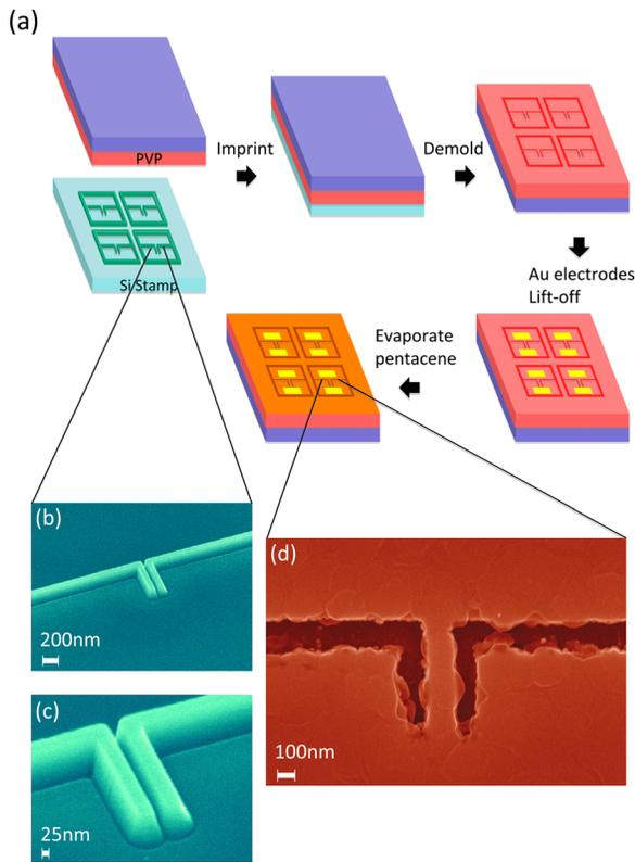
FIG. 1. (Color online) (a) Schematic of process flow for fabricating organic in-plane diodes. (b) SEM image of  $W = 25$  nm,  $L = 500$  nm Si stamp (c) Magnified SEM image of  $W = 25$  nm,  $L = 500$  nm Si stamp (d) SEM image of  $W = 150$  nm,  $L = 500$  nm finalized device.
