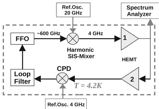
**Fig. 11.3** Flow chart of the CPLL for FFO phase locking
