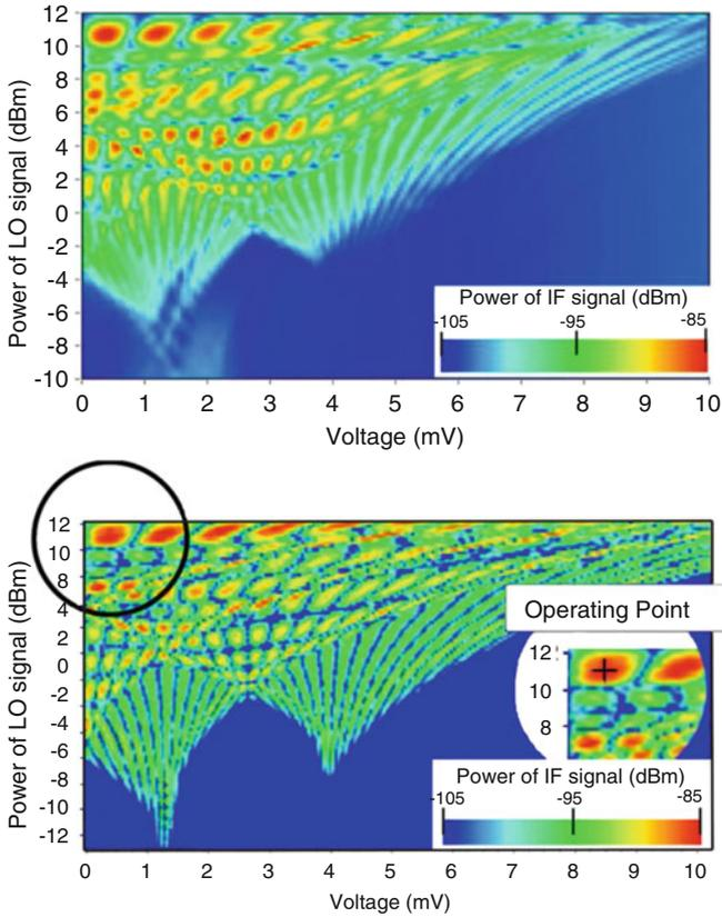
**Fig. 11.7** Experimental (*up*) and theoretical (*bottom*) dependence of IF signal's power versus LO signal's power and bias voltage across the HM. The operating point with the maximum power of IF signal ( $-85$  dBm) is shown on the theoretical dependence. The FFO frequency is 636 GHz, LO frequency – 18 GHz (the 35th harmonic of LO is used) as result frequency of IF signal is equal 6 GHz. The critical current of the SIS junction was suppressed by the magnetic field
