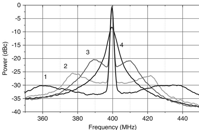
**Fig. 11.4** Downconverted spectra of the FFO operating at 600 GHz: curve “1” – Free running, linewidth 2 MHz; “2” – phase-locked with CPLL, BW 40 MHz (SR = 93.5%); “3” – phase-locked with CPLL, BW 25 MHz (SR = 90.5%); “4” – phase-locked with RT PLL, BW 12 MHz (SR = 82%)
