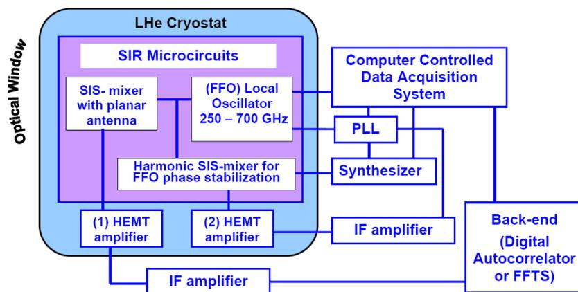
Figure 1. Block-diagram of the superconducting integrated receiver.
