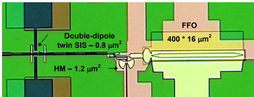
Figure 4. Central part of the SIR chip with double-dipole antenna, twin SIS-mixer and harmonic mixer for FFO phase locking.
