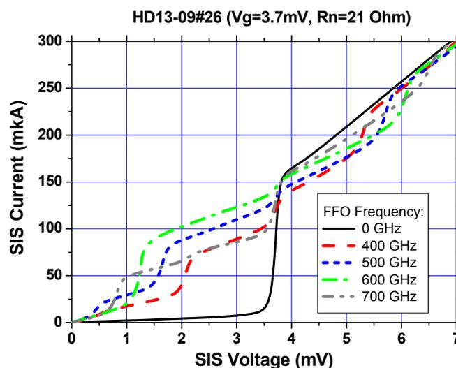
Figure 2. IVCs of the SIS mixer: unpumped – solid curve, pumped at different frequencies – dashed and dotted lines<sup>15</sup>.
