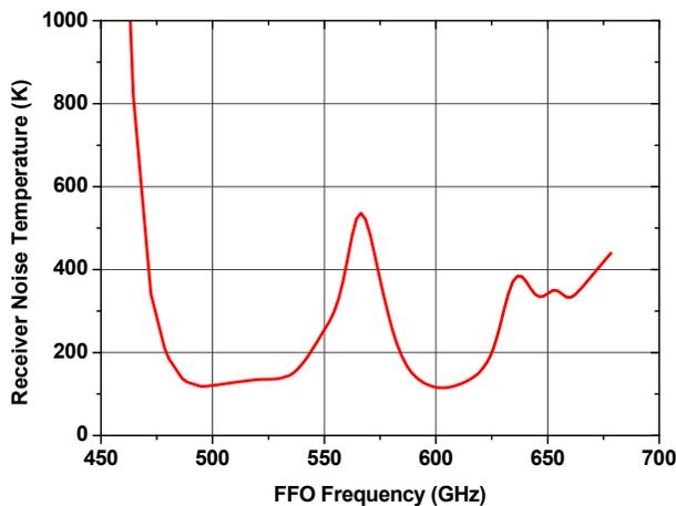
Figure 5. Measured DSB receiver noise temperature of the SIR for the flight device at IF frequency 8 GHz.
