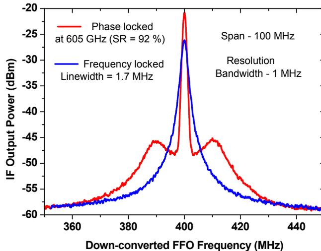
Figure 3. Spectra of the Nb-AlN-NbN FFO operating at 515.2605 GHz (blue curve – frequency locked by FD; red curve – phase-locked). Linewidth = 1.7 MHz; Spectral Ratio = 92 %.
