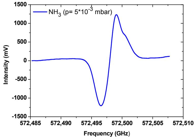
Figure 12. Response (derivative of the spectral line), measured for  $\text{NH}_3$  gas by the integrated receiver with implementation of novel technique (details will be published elsewhere).
