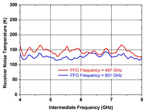
Figure 6. DSB receiver noise temperature as a function of the IF frequency, taken at two FFO frequencies: 497 and 601 GHz.
