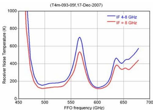
Fig. 7 Measured DSB receiver noise temperature of the SIR device selected for flight at 8 GHz IF frequency (red line) and integrated in the 4-8 GHz IF range (blue curve)
