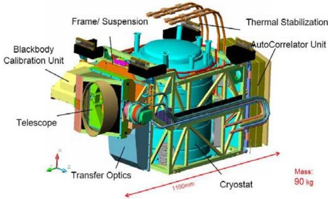
Fig.2 Design drawing of the complete TELIS instrument
