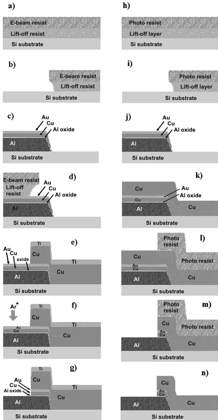
FIG. 1. Comparison between the two versions of the fabrication procedure: Technology 1 (column to the left); Technology 2 (column to the right).
