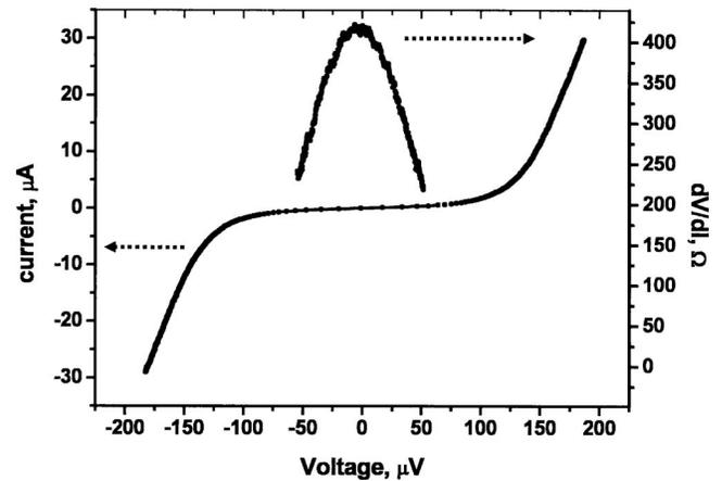
FIG. 5. *IV* curves and  $dV/dI$  at 300 mK, Technology 2.
