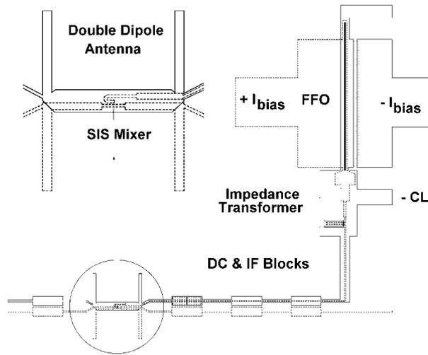
**Figure 1.** Schematic of the SIR chip. Planar antenna coupled SIS mixer is pumped by an integrated on the same chip Local Oscillator - Flux Flow Oscillator (FFO).
