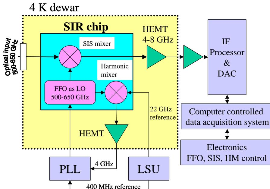
**Figure 2.** PLL configuration of the HM option. Planar antenna coupled SIS mixer is pumped by an integrated FFO. A small fraction of the FFO is directed towards the HM. The latter mixes the FFO with the  $n$ -th harmonic of the 22-24 GHz reference standard signal. Frequency and phase of the mixing product are compared in the PLL system with the reference 400 MHz. Finally, the phase difference signal generated by the PLL is used to feedback the FFO bias to compensate for the phase error.
