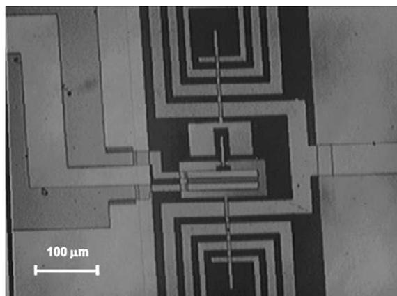
Fig. 3. Photo of high- $T_c$  dc SQUID RF amplifier with gradiometric configuration.
