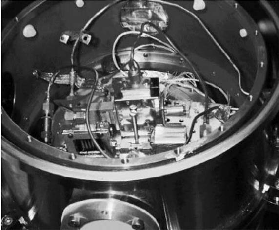
Fig. 5. Inside of the helium cryostat with SQUID and filter installed.
