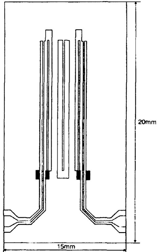
Fig. 1. Layout of a three-pole co-planar waveguide filter.
