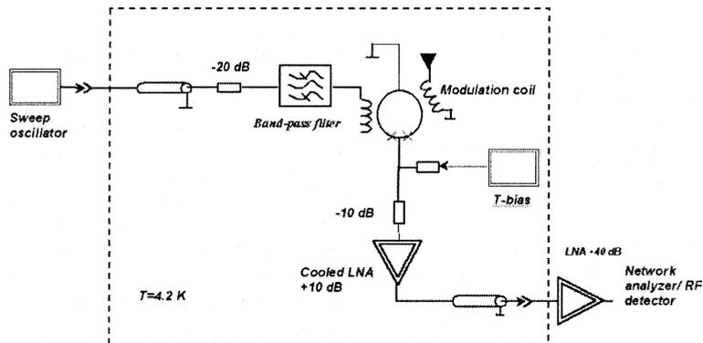
Fig. 6. Schematics of the measurements system.
