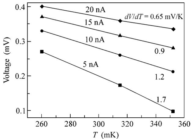
**Fig. 3.** Temperature dependences of the voltage on bolometer for various bias currents.
