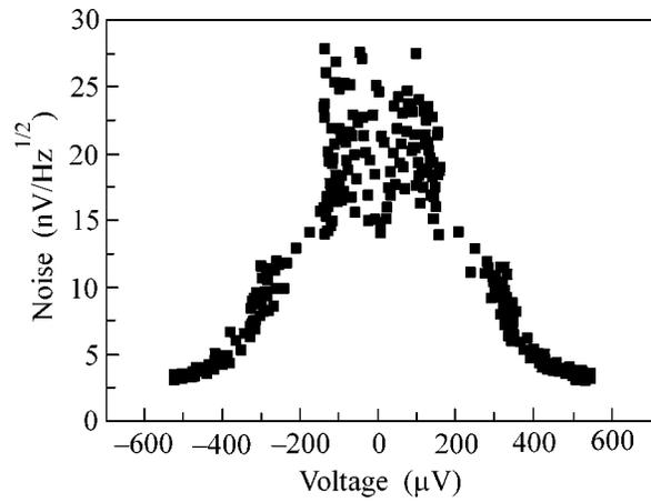
**Fig. 5.** Dependence of the noise in the range 1–10 kHz on the bias voltage on a bolometer with 30 nm chromium and 30 nm aluminum. At biases higher than 500  $\mu\text{V}$ , noise is restricted by the amplifier.
