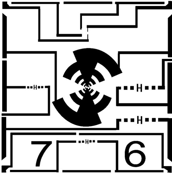
**Fig. 1.** Microphotograph of a bolometer chip with 16 contact pads and six CCHNEB structures. Log-periodic antenna is at the center; two double dipole antennas for the central frequency 300 GHz are on the right and two antennas for 600 GHz are on the left and at the bottom.
