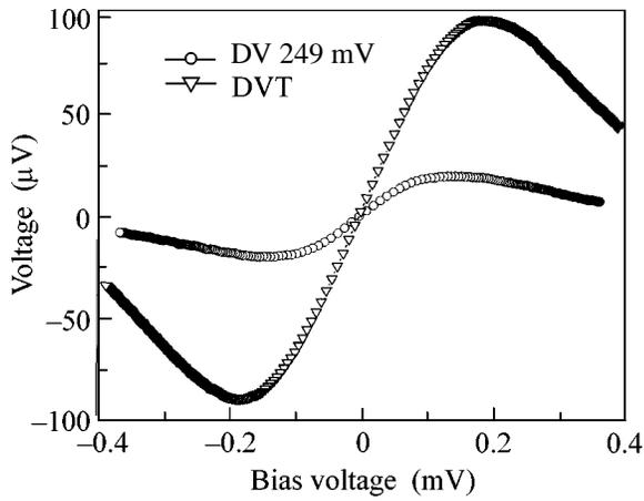
**Fig. 4.** CCHNEB voltage response (curve DVT) to a change in temperature and (curve DV 249 mV) to the black-body radiation.
