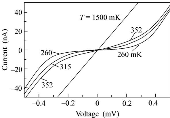
**Fig. 2.** Current–voltage characteristics of bolometer, as measured at temperatures from 260 mK to 1.5 K.
