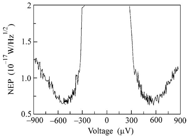
**Fig. 6.** Noise-equivalent power measured for the sample with 30 nm Cr and 30 nm Al in the absorber film.
