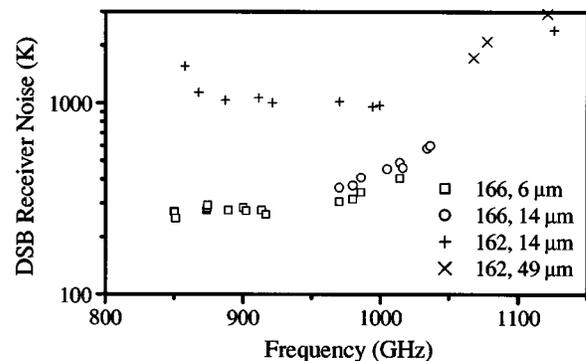
FIG. 4. DSB receiver noise temperatures of mixers 162 and 166 as a function of frequency. Mixer 166 is measured at 2.9 K using 6 and 14  $\mu\text{m}$  beamsplitters, while mixer 162 is measured at 4.6 K with 14 and 49  $\mu\text{m}$  beamsplitters and a thick vacuum window (100  $\mu\text{m}$  Mylar™).
