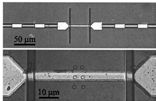
FIG. 1. Optical microscope images of the twin-slot antenna and double-junction tuning structure used here. The SIS junctions are  $\sim 1 \mu\text{m}^2$ .
