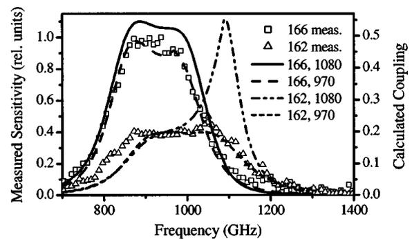
FIG. 3. Direct detection response measured in vacuum at 4.6 K for mixers 166 and 162, with  $1.05$  and  $0.70 \mu\text{m}^2$  junctions, respectively. Also shown are the predicted responses of each mixer, assuming NbTiN gap frequencies of 970 and 1080 GHz. The observed drop in device sensitivities at  $\sim 1$  THz is attributed to increasing loss in the NbTiN.
