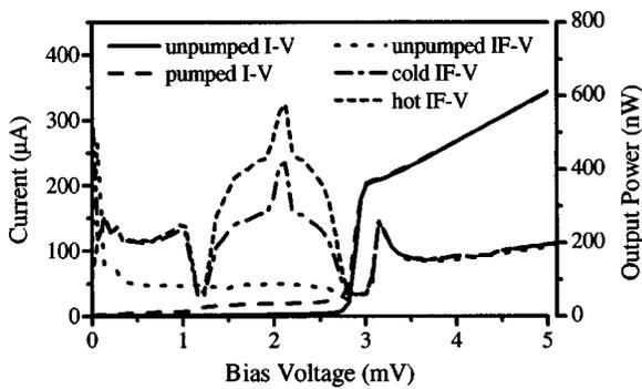
FIG. 2. Bias current and IF output power vs bias voltage for a device measured at 2.9 K with and without 980 GHz local oscillator power. For the pumped measurements, the IF output is measured for 77 and 295 K signal sources, yielding a DSB receiver noise of 315 K at  $\sim 2.3$  mV.
