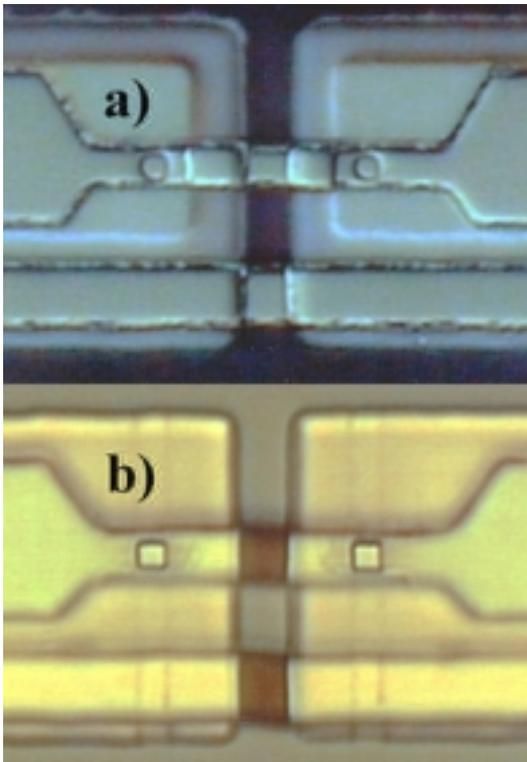
Fig. 3 Examples of definition of SIS junction for balanced mixer [3], [4]: single step windows (a) and cross-bar windows (b) The area of junctions is about 2 micrometers; alignment accuracy is better than 0.5  $\mu\text{m}$ .
