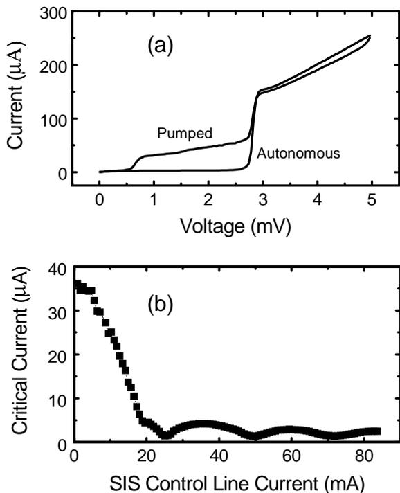
Fig. 5 Main characteristics of the SIS mixer: IV-curves, autonomous and pumped by FFO at 500 GHz (a) and control line characteristic (b).
