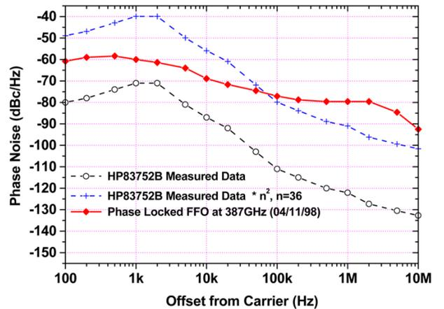
**Figure 6.** Experimentally measured phase noise of the phase locked FFO at 387 GHz compared with the data for an HP83752B synthesizer [28]. Since the residual phase noise of the FFO is measured relative to the 36th harmonic of the synthesizer, a multiple factor of  $36^2 = 1296$  has to be used to estimate the total FFO phase noise.
