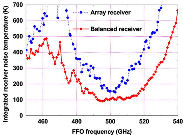
**Figure 12.** Circles, experimental data on a typical single-junction pixel pumped by its internal FFO in a nine-pixel array cryostat. The data are collected automatically by the IRTECON system; ripples are associated with interference on a thick 80 K infrared filter. Diamonds, data on a pixel with the double-junction *balanced SIS mixer* pumped by the integrated FFO measured in a smaller test cryostat.
