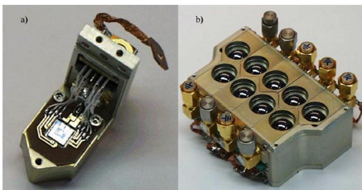
**Figure 15.** (a) Replaceable element of the nine-pixel imaging array. The unit is shown from the side of the receiver chip, which is mounted on the elliptical microwave lens and wire bonded to the printed circuit board. (b) Nine-pixel imaging array receiver block. Each pixel is an independent integrated receiver with its own internal local oscillator. The array mount is shown from the side of its input microwave lenses.
