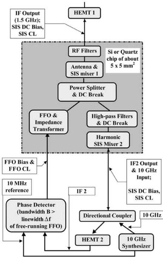
**Figure 14.** Block diagram of the proposed sub-millimetre all-superconducting phase locked single-chip integrated receiver [49]. The common FFO pumps two SIS mixers: one serves as the detector/mixer, and the other facilitates the phase locking of the FFO.
