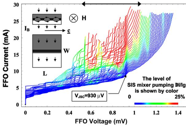
**Figure 1.** IVCs of the Nb–AlO<sub>x</sub>–Nb FFO recorded at different magnetic fields produced by an integrated control line. Note an abrupt changing of the IVC at boundary voltage  $V_{JSC} \approx 930 \mu\text{V}$ . Inset, cross section of the long junction with driven vortices (top) and its layout (bottom). Here  $I_B$  is bias current;  $L$  and  $W$  are length and width of the FFO respectively.
