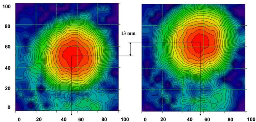
**Figure 17.** Antenna beam pattern for two adjacent pixels; contour steps are at 1 dB. Both axes present the linear shift of the irradiation source (in millimetres). The antenna beam is mapped at 470 GHz with the source in front of the test Dewar at the distance of 40 cm.
