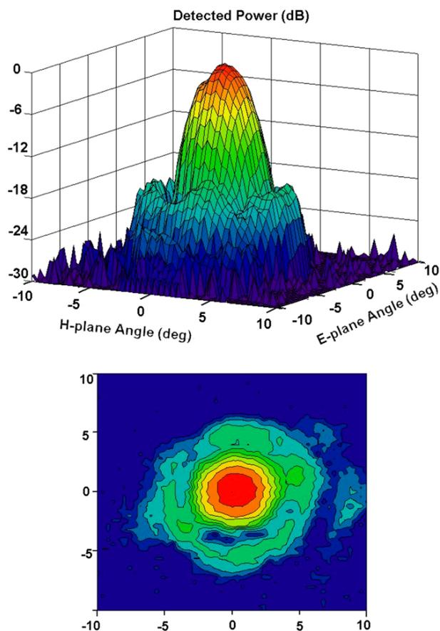
**Figure 13.** Antenna beam pattern of the SIR pixel measured at the distance of 400 mm from the cryostat window at 490 GHz. Data for the raster image are collected from an area 100 mm by 100 mm. The equal power contours are placed with steps of 3 dB. The first sidelobe is found at  $-16$  dB. Some asymmetry is assumed to be a result of sidelobes touching the shielding can.
