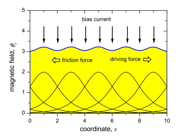
$$V_{\rm FF} = \frac{\Delta\Phi}{\Delta t} = \frac{H\Lambda L}{L/u} = H\Lambda u$$
