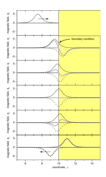
Collision with edge  $\equiv$  fluxon-antifluxon collision
