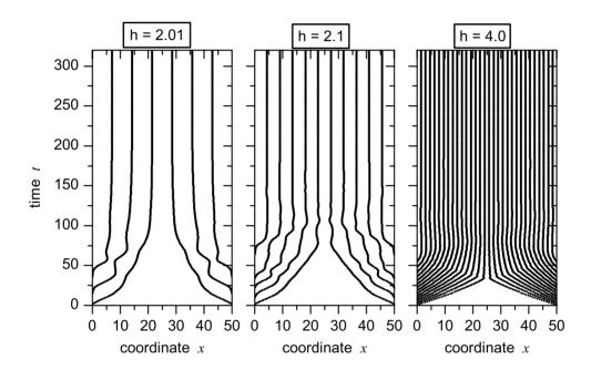
Example: h=4,  $\phi=hx$ , so  $\phi(L)-\phi(0)=h\ell$ ,  $N=\frac{h\ell}{2\pi}=\frac{4\times50}{6.28}\approx31.8$ . Looking at picture, we see 30 fluxons. For smaller fields the correspondence is worse, since the dense fluxon chain approximation works not so good, and at h<2 does not work at all. e.g. for h=2.1, N=16.7, but we see only 10 fluxons.
